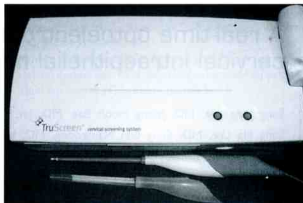
Fig. 1. The appearance of TruScreen. TruScreen is a portable system which consists of a console and a pen-shaped probe. The size of the console is 38×19×7 cm and the length of the disposable white cap is 25 cm.
